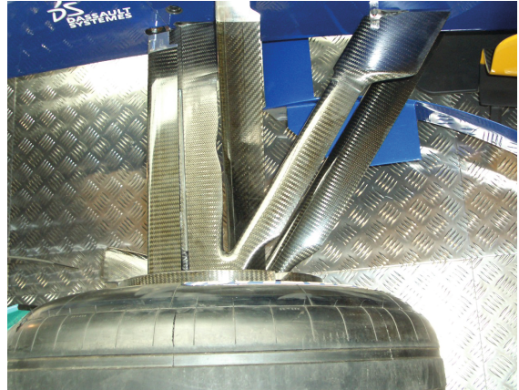
Wheel suspension made from CFC (carbon fiber composite) (photo by Julian Eichhoff)
