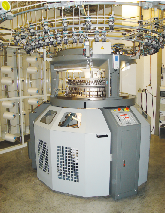
Figure 5.14 Circular knitting machine (Courtesy of Beck)
