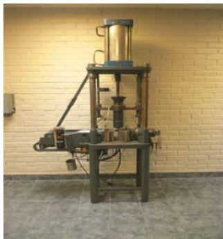
Fig 194. The picture shows an old piston injection-molding machine. The locking mechanism was a knee-joint type that is commonly used even today, but the locking and opening movements required arm muscles to operate the levers.
