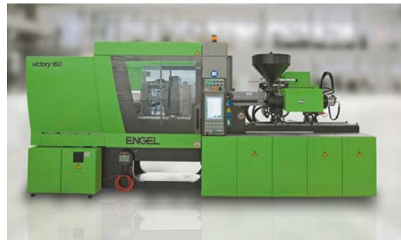
Fig 195. A modern injection-molding machine manufactured by Engel. This machine has a hydraulic locking mechanism. You can also get "all-electric" machines, which are significantly quieter than the hydraulic ones. Photo: Engel
