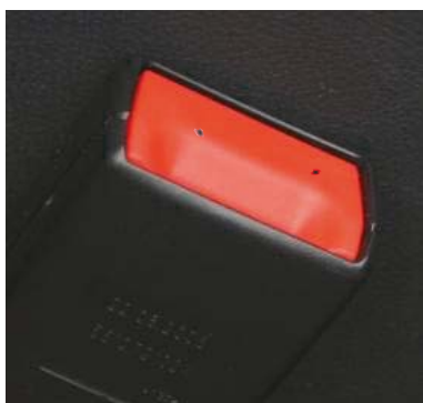
Fig 507. The black specks that you can see on the red button of the safety belt lock are an unacceptable deviation. It is normally defined as a surface defect.
