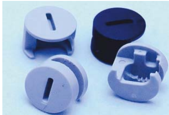
Fig 264. Here we can see a common component used in assembly of furniture. AD-Plast in Sweden developed this component in PPA with glass. They won the prestigious price “Plastovationer 2009” by successfully replacing metal with plastic. The cam is stronger than the former zinc one without needing to change the outer dimensions. Source: AD-Plast AB
