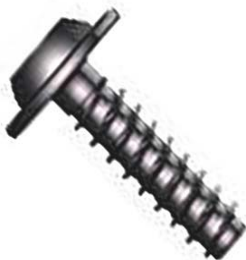
Fig 434. If a good screw joint is required for a self-tapping screw, the plastic material should have a stiffness lower than 2800 MPa (i.e. the same as for POM). For stiffer materials (e.g. glass fiber reinforced), a threaded hole or threaded inserts are recommended. It is also important to use a self-tapping screw that is specifically developed for plastic materials.
