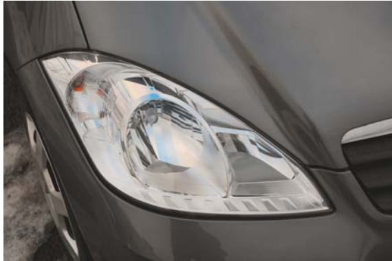
Fig 211. A headlamp housing made in PBT
