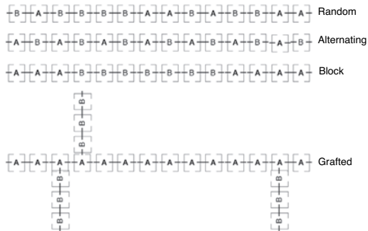
Figure 2.2: Schematic representation of different copolymers.
